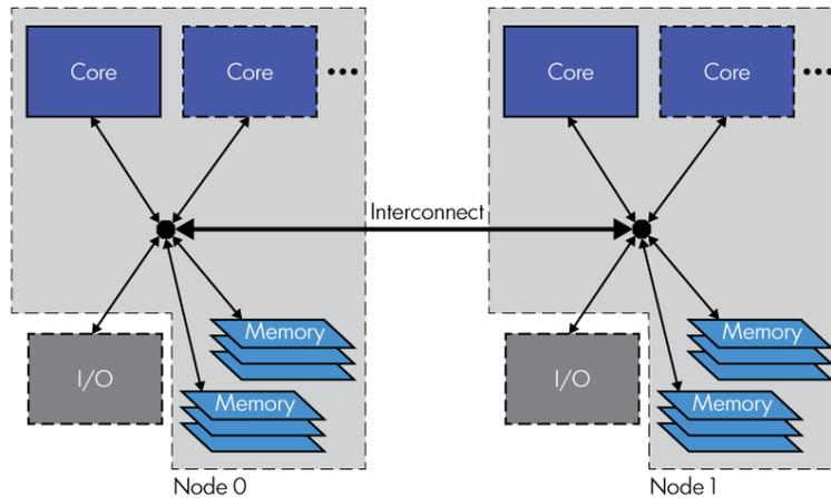
Ideally, the intranode core-to-memory and I/O-to-memory bandwidths are sufficient to handle (1) the requirements of the cores and the I/O subsystems contained within each node and (2) incoming accesses from remote nodes. If the intranode bandwidth is insufficient for the node's core and I/O requirements, the server suffers from the same bottlenecks within a node that the NUMA implementation is intended to address at the system level.
