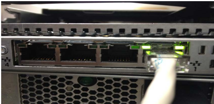
Figure 1 Quad-port LOM on a ProLiant DL360p Gen8 server. The ports are labeled right to left
