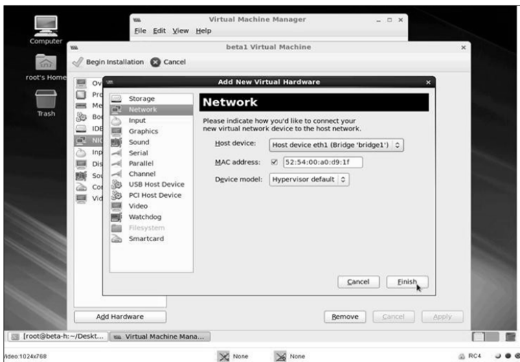
FIGURE 10. virt-manager window to add new network interface on guest
