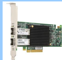
CN1200E Dual Port Converged Network Adapter
