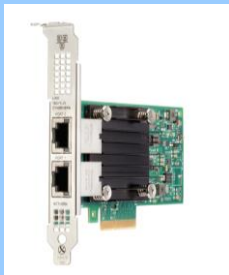
HPE Ethernet 10Gb 2-port BASE-T X550-AT2 Adapter
