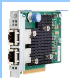
HPE Ethernet 10Gb 2-port FLR-T X550-AT2 Adapter
