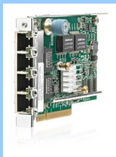
HPE Ethernet 1Gb 4-port FLR-T I350-T4V2 Adapter
