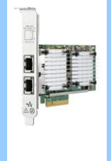
Ethernet 10Gb 2-port BASE-T Adapter
