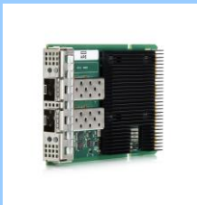
Ethernet 10/25Gb 2-port SFP28 OCP3 Adapter
