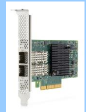
Ethernet 10/25Gb 2-port SFP28 Adapter
