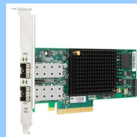
HP CN1000E Dual Port Converged Network Adaptor
